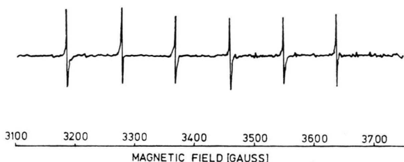
Fig. 2a. Hyperfine splitting of ^{55}\text{Mn}^{2+} in chromium doped forsterite. The spectrum was taken at room temperature and 9.527 GHz. The crystal was oriented with a \perp H_0 .
